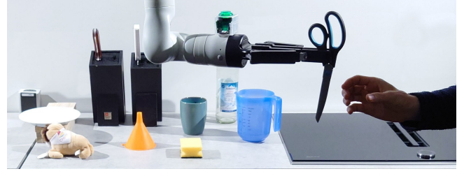
Figure 2: Close-up of the study setup. Participants stand at one of two approach positions facing the robot arm. When the robot stops moving, participants can press the green button to confirm the end of the handover.
